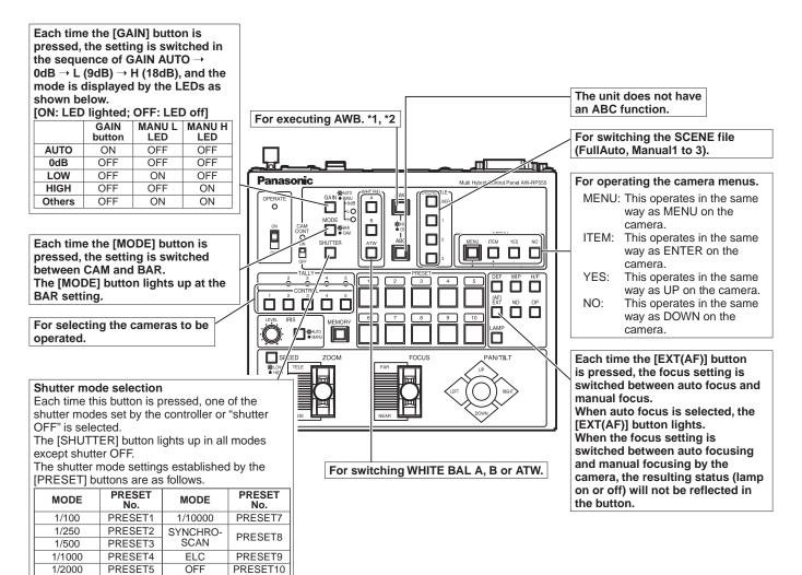
\*1: The lamp of the AWC switch flashes while automatic white balance is being executed. When AWB is completed successfully, the lamp goes off; when it is not completed successfully, it lights up.
